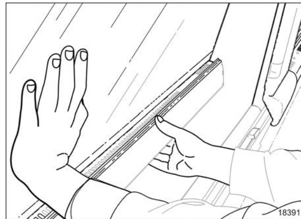
FIGURE 16: EMERGENCY WINDOW OPENING
