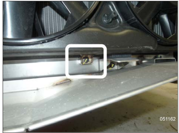
FIGURE 11: FAN SHROUD TOP & BOTTOM HOLD-DOWN SCREWS
