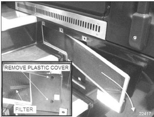
FIGURE 21: REMOVING DRIVER'S SECTION AIR FILTER
