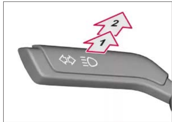
FIGURE 25: HIGH BEAM CONTROL
