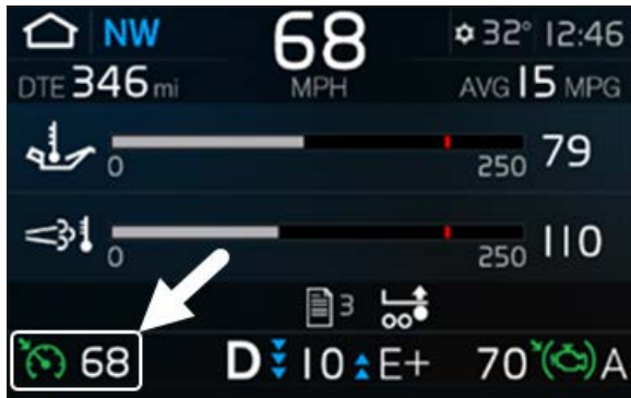
FIGURE 38: CRUISE CONTROL SET SPEED CONFIRMATION & CURRENT SET SPEED DISPLAYED IN THE SYSTEM STATUS ZONE
