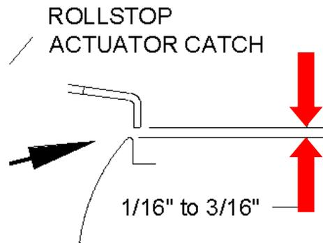
FIGURE 4-21: ROLLSTOP ACTUATOR
