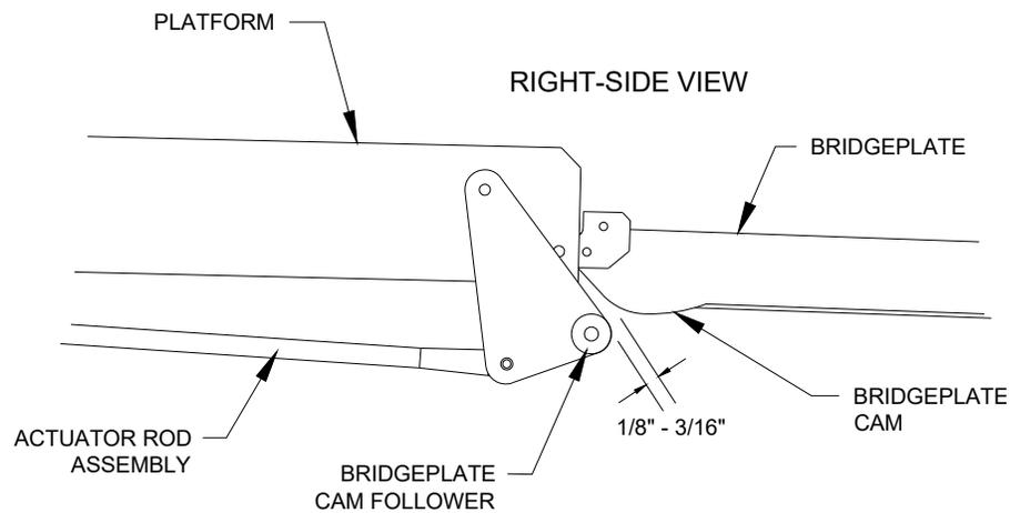
**FIGURE 2-4: BRIDGEPLATE ADJUSTMENT**
