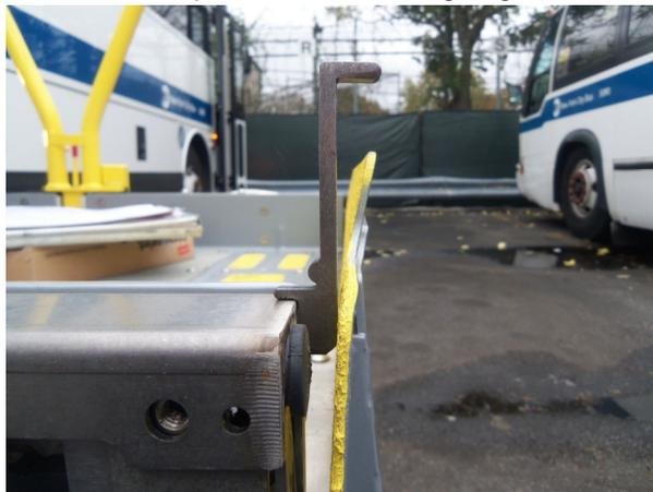
**FIGURE 4-24: ROLLSTOP ADJUSTMENT TOOL P/N 55273**
