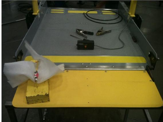
**FIGURE 2-7. 25 LBS. (11 KG) LOAD TEST (LEFT SIDE)**
