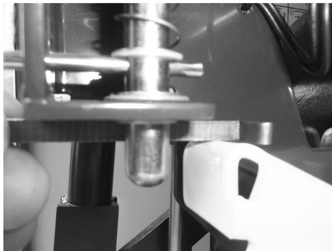
FIGURE 4-43C: VERIFY GAPS WITH TOOL P/N 55273
