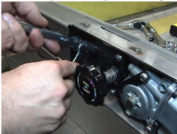
FIGURE 4-11: LOOSEN JAM-NUT
