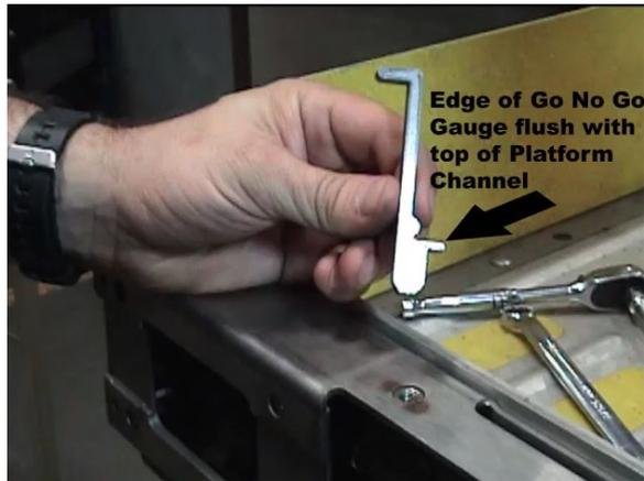
**FIGURE 4-5: ROLLSTOP ADJUSTMENT TOOL P/N 55273**
