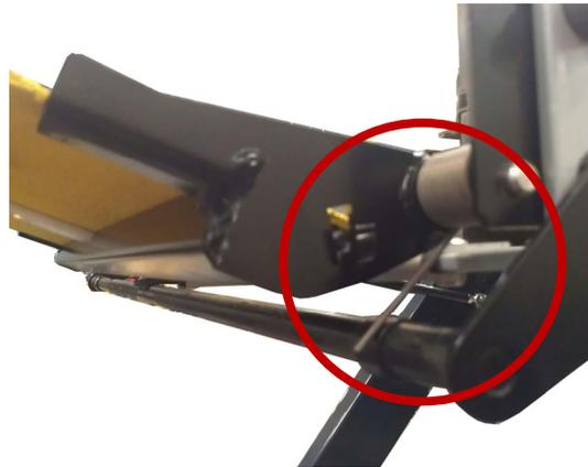
**FIGURE 2-10. UNHOOK BRIDGEPLATE SPRING**
