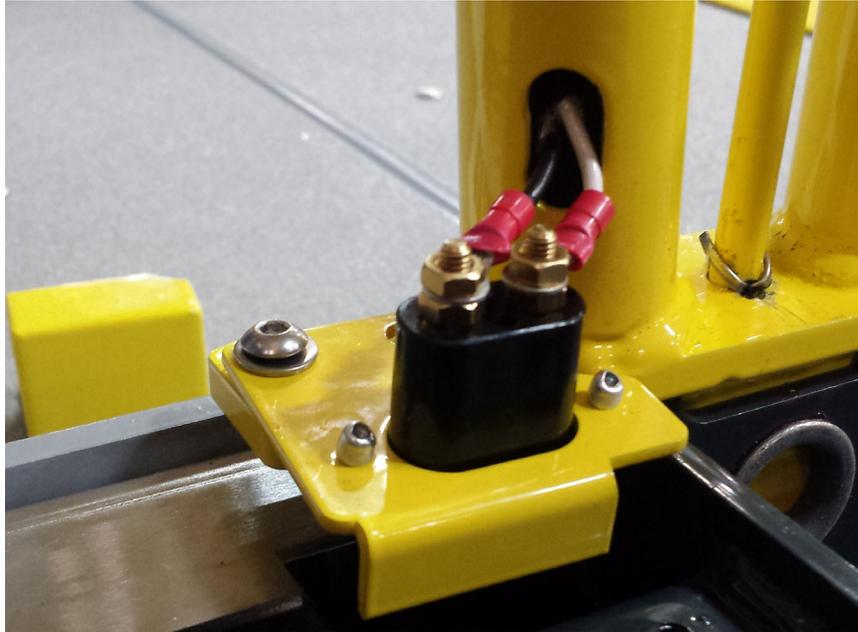
FIGURE 4-49: CONTACT SWITCH
