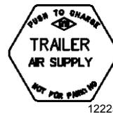
The trailer air braking system is supplied by pushing this control valve.
