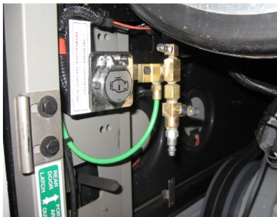
FIGURE 23 : ENGINE COMPARTMENT EMERGENCY AIR-FILL VALVE
