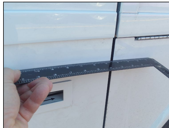
FIGURE 67: USE A RULER (SHOWN IN BLACK) TO CHECK THAT SURFACES ARE EVEN
