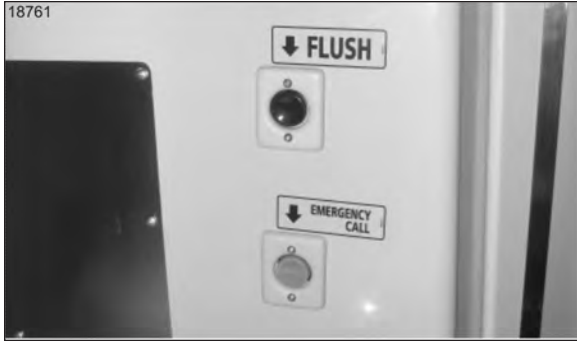
FIGURE 21: FLUSH AND EMERGENCY BUTTONS
