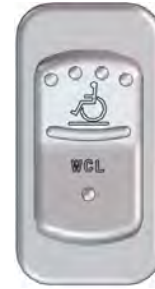
FIGURE 9: WHEELCHAIR LIFT POWER SWITCH
