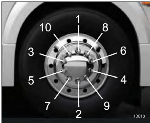
FIGURE 13: TIGHTENING SEQUENCE
