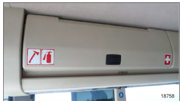
FIGURE 8: A DECAL INDICATES THAT A FIRE HATCHET, A FIRE EXTINGUISHER AND A FIRST-AID KIT ARE LOCATED IN THIS OVERHEAD COMPARTMENT
