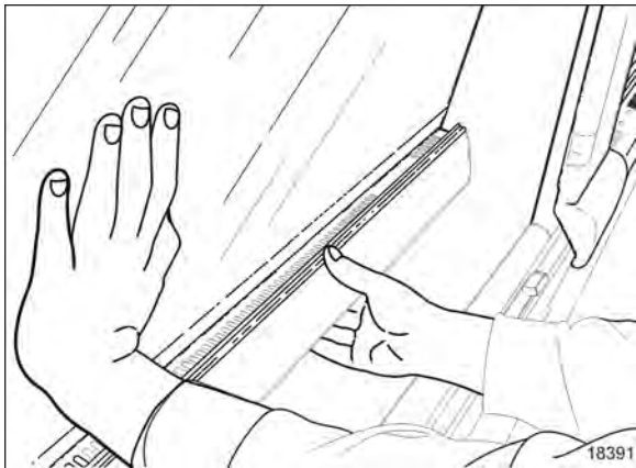
FIGURE 14: EMERGENCY WINDOW OPENING
