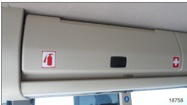
FIGURE 9: A DECAL INDICATES THAT A FIRE EXTINGUISHER AND A FIRST-AID KIT ARE LOCATED IN THIS OVERHEAD COMPARTMENT
