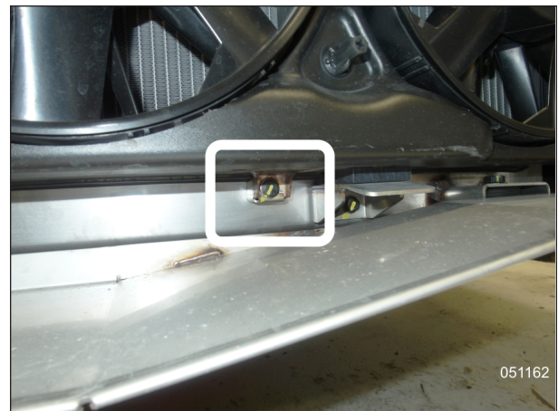
FIGURE 13: FAN SHROUD TOP & BOTTOM HOLD-DOWN SCREWS
