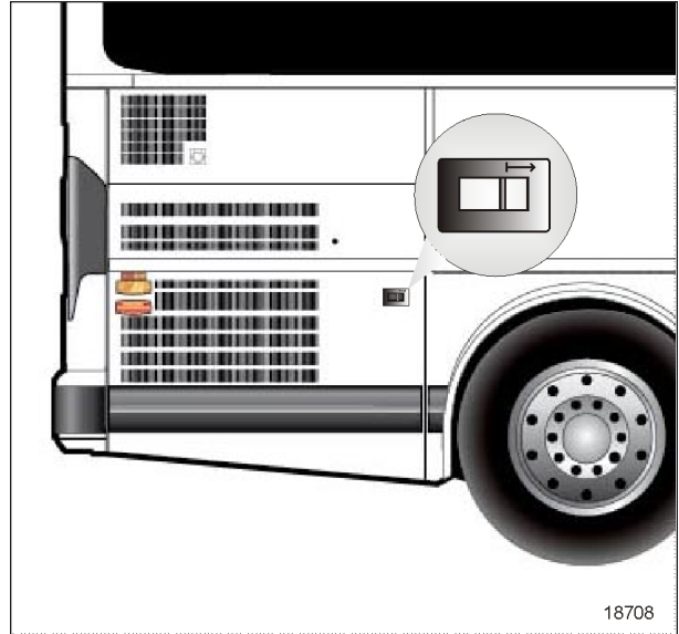
FIGURE 6: ENGINE COMPARTMENT CURBSIDE DOOR
