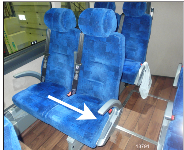
FIGURE 9: PULL TO UNLOCK THE ROTATION
