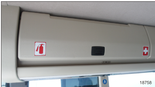
FIGURE 10: A DECAL INDICATES THAT A FIRE EXTINGUISHER AND A FIRST-AID KIT ARE LOCATED IN THIS OVERHEAD COMPARTMENT
