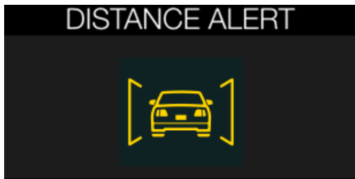
FIGURE 50: FOLLOWING DISTANCE ALERT WARNING POP-UP
