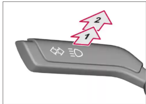
FIGURE 26: HIGH BEAM CONTROL
