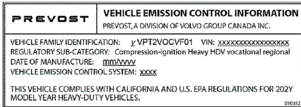
Figure 1: Vehicle Emission Control Information label sample
