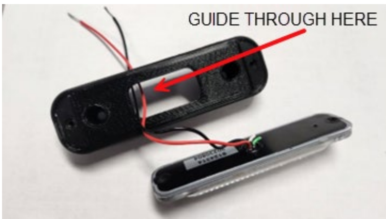
Figure 7: Red and black wires guided through the TWS light adapter
