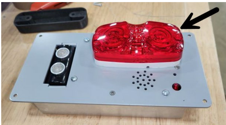
Figure 1 : Red lens cover to be removed
