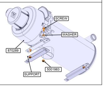
23. Install the new heater assembly.
