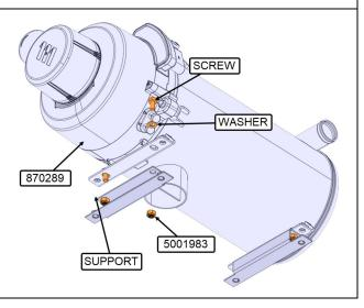
23. Install the new heater assembly.
