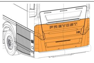
73. Close the compressor door. The procedure is complete, no further actions required.
