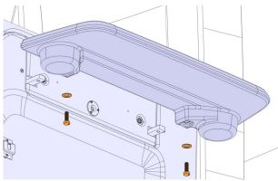
3. Remove the screws (2x) and the panel.
