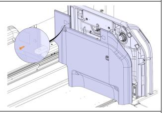
4. Slide the dam plate 3202286 between the floor and the modesty panel structure.
