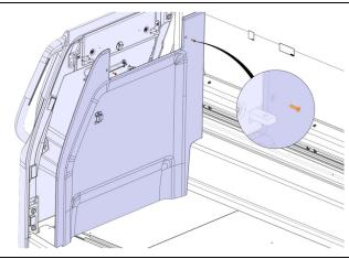
4. Slide the dam plate 3202287 between the floor and the modesty panel structure.
