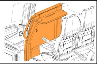
2. Remove the nuts (2x) and the washers (2x) and remove the shelf.
