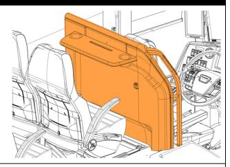
2. Remove the nuts (2x) and the washers (2x) and remove the shelf.
