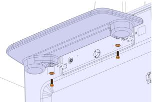
3. Remove the screws (2x) and the panel.
