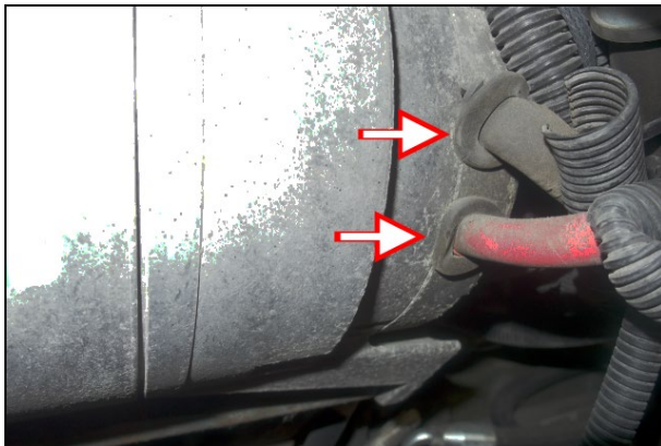
Figure 24: Bosch T1 alternator with the two required rubber grommets. Alternator cables connected to the alternator stud terminals must be protected against metal edges with rubber grommets.
