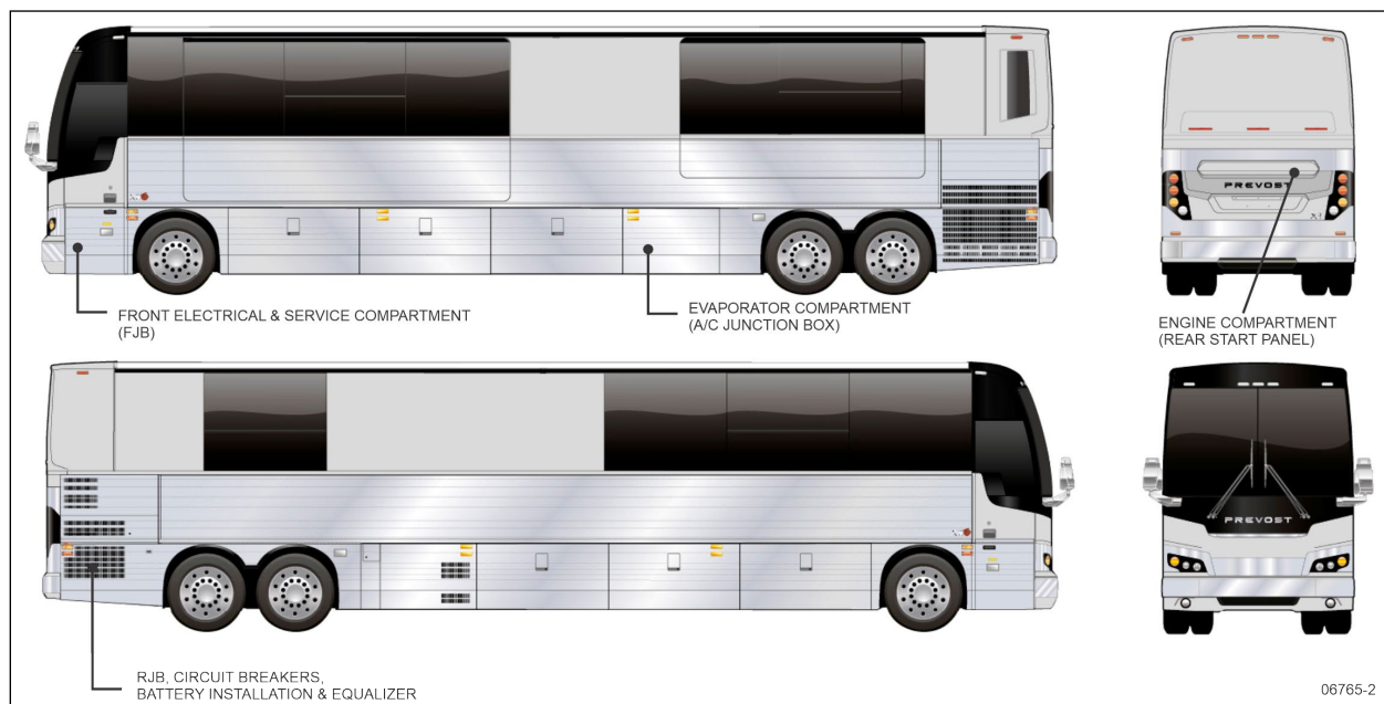
FIGURE 19: ELECTRICAL COMPARTMENTS (X3-45 VIP)
