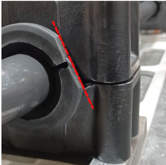
FIGURE 9: RESPECT THE ORIENTATION OF THE FLAT ON THE SPLIT BUSHING IN RELATION WITH THE CLAMP HALVES
