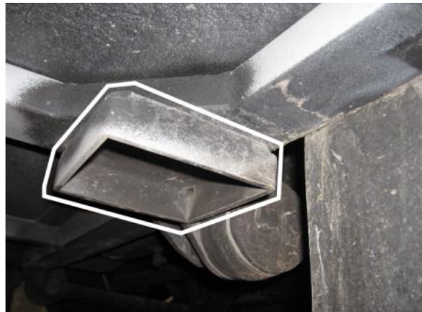
FIGURE 17 : OPTIONAL CHASSIS HOISTING RECEPTACLES - AFT OF FRONT AXLE
