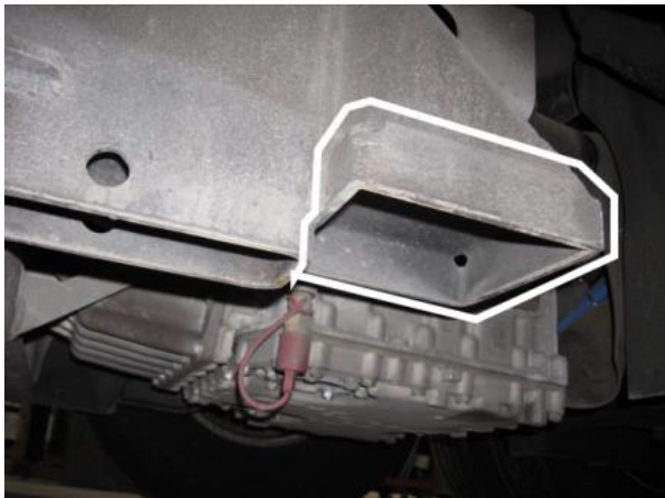
FIGURE 16 : OPTIONAL CHASSIS HOISTING RECEPTACLES - AFT OF TAG AXLE
