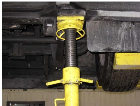
FIGURE 19 : JACK STAND AT CHASSIS HOISTING RECEPTACLE - AFT OF FRONT AXLE, CURB SIDE
