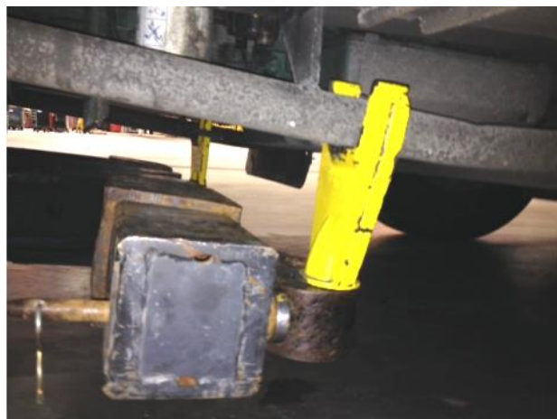
FIGURE 62 : PROPER LOCATION WHEN LIFTING THE SIDE MEMBERS
