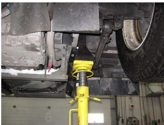
FIGURE 20 : JACK STAND AT CHASSIS HOISTING RECEPTACLE – AFT OF TAG AXLE, ROAD SIDE
