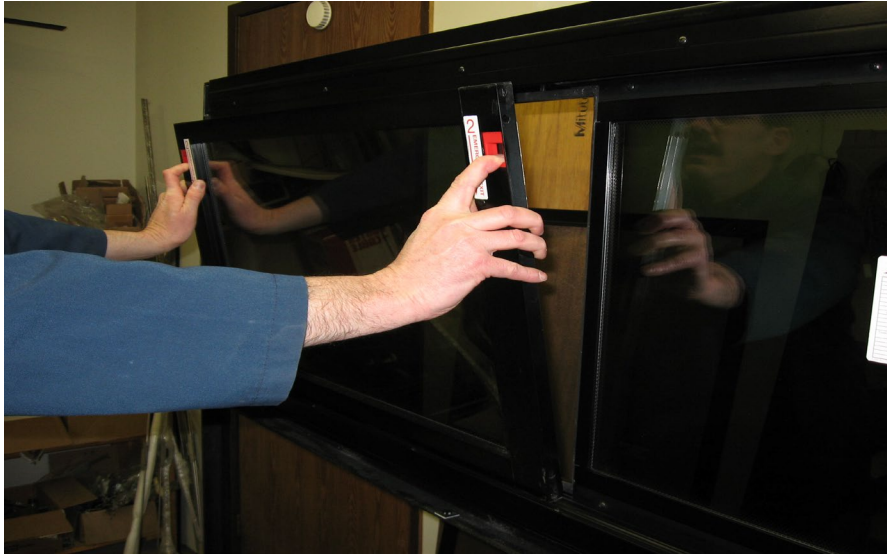
FIGURE 47: REMOVING THE SASH
