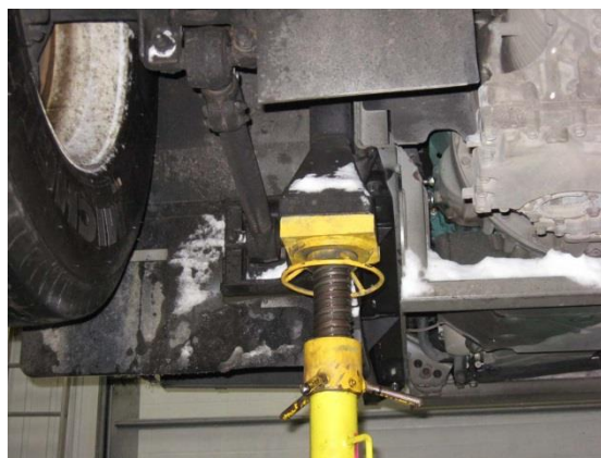
FIGURE 21 : JACK STAND AT CHASSIS HOISTING RECEPTACLE – AFT OF TAG AXLE, CURB SIDE
