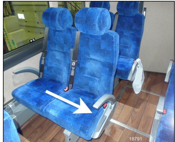
FIGURE 32: PULL TO UNLOCK THE ROTATION
