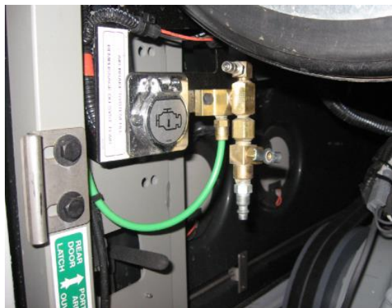
FIGURE 24 : ENGINE COMPARTMENT EMERGENCY AIR-FILL VALVE
