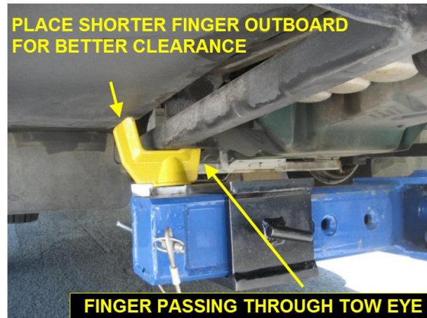
FIGURE 63 : PROPER LOCATION WHEN LIFTING THE SIDE MEMBERS – VEHICLE EQUIPPED WITH REAR TOW EYES
