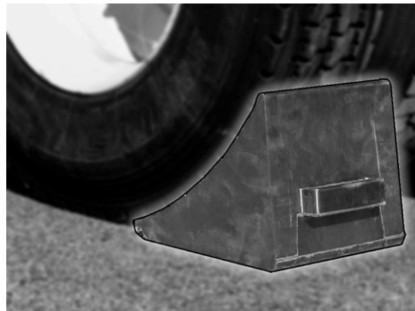
FIGURE 22 CHOCK THE FRONT AND REAR WHEELS
