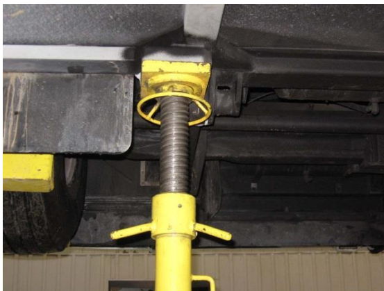
FIGURE 18 : JACK STAND AT CHASSIS HOISTING RECEPTACLE - AFT OF FRONT AXLE, ROAD SIDE
