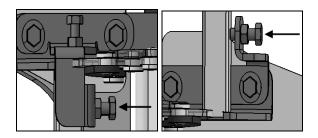
5. To adjust door depth, loosen the screws fixing the hinge to frame assembly and slide the hinge horizontally to move the door in or out. Depth should be calculated at 29mm +/2mm measured from bus frame out or 5mm +1mm if measurement is taken from small square tube on frame.
