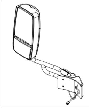
FIGURE 25: REAR VIEW MIRROR (ROSCO) 18398B
