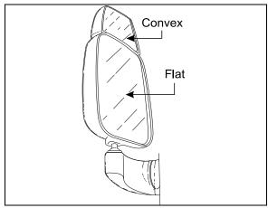
FIGURE 15: REAR VIEW MIRROR (RAMCO)
