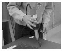
7. Once the welding torch is ready, insert the filler bead into the nozzle and immediately start welding. Move in a regular manner while pressing slightly with torch.
