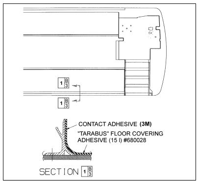
FIGURE 93: TARABUS FLOOR COVERING ADHESIVE APPLICATION
