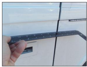
FIGURE 67: USE A RULER (SHOWN IN BLACK) TO CHECK THAT SURFACES ARE EVEN
