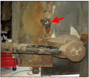
FIGURE 6: CLEANED SPOT ON STRUCTURAL MEMBER
