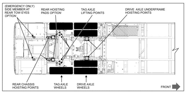
FIGURE 15: X-SERIES OPTIONAL REAR CHASSIS HOISTING POINTS
