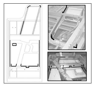
> Apply some #680066 glue inside fiber glass groove and fix power window wiper.
