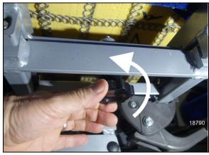
FIGURE 88: LOOSEN THE KNOB
