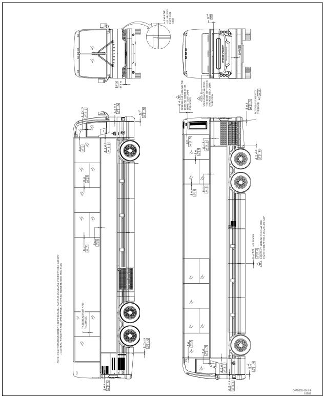
FIGURE 150: BODY PANEL & WINDOW SPACING FOR X3-45 VIP NOT FITTED WITH SLIDE-OUT
