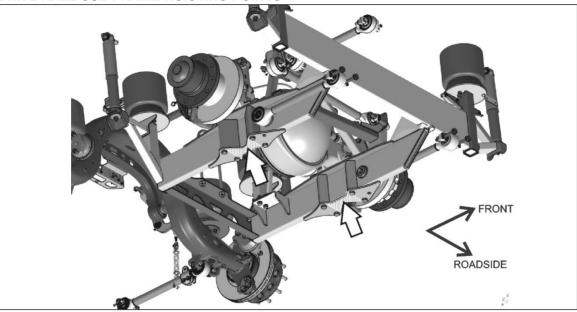
FIGURE 12: DRIVE AXLE SUB FRAME HOISTING POINTS.
