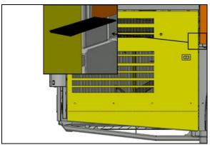
FIGURE 133: USE A RULER (SHOWN IN BLACK) TO CHECK THAT SURFACES ARE EVEN
