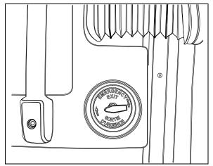
FIGURE 25: INTERIOR UNLATCH AIR VALVE
