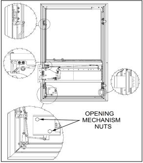
FIGURE 80: WCL SLIDING DOOR OPENING MECHANISM 18740
