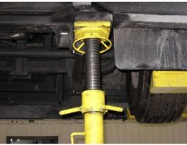
FIGURE 19: JACK STAND AT CHASSIS HOISTING RECEPTACLE - AFT OF FRONT AXLE, CURB SIDE
