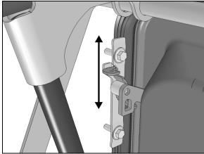
Make sure that skid bar only touches slightly bus structure at bottom. The door should not move up when closing.
