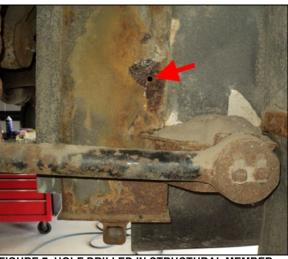
FIGURE 7: HOLE DRILLED IN STRUCTURAL MEMBER
