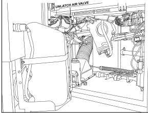
FIGURE 26: EXTERIOR UNLATCH AIR VALVE 12209
