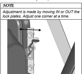
5. Check handle adjustment. Handle must remain tight against its plastic housing.
