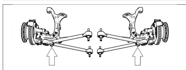
FIGURE 10: INDEPENDENT FRONT SUSPENSION (IFS) PREVIOUS DESIGN - HOISTING POINTS
