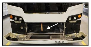
FIGURE 13: FRONT BUMPER AND SPARE TIRE
