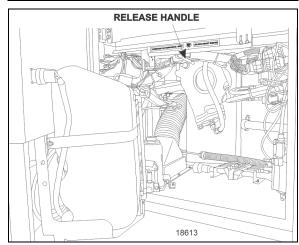
FIGURE 12: FRONT BUMPER RELEASE HANDLE 18613
