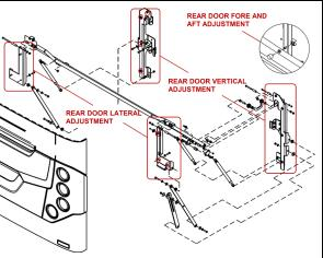
FIGURE 47: ENGINE COMPARTMENT DOOR
