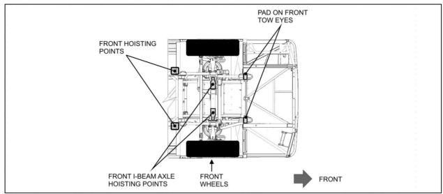
FIGURE 14: OPTIONAL FRONT CHASSIS HOISTING POINTS
