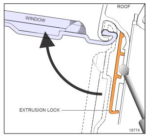
FIGURE 42: EMERGENCY EXIT WINDOW REMOVAL
