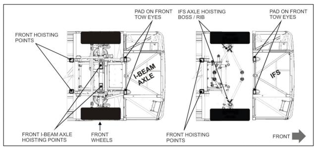
FIGURE 1 FRONT HOISTING AND LIFTING POINTS DIAGRAM
