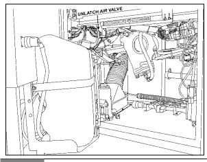
FIGURE 35: EXTERIOR UNLATCH AIR VALVE 12209
