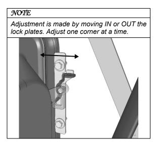
15. Check handle adjustment. Handle must remain tight against its plastic housing.
