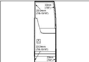
FIGURE 29: SEAL COMPRESSION ADJUSTMENT 1863:
