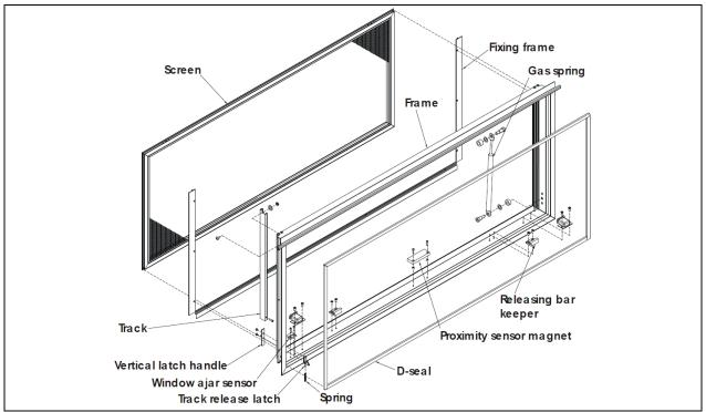
FIGURE 105: ELECTRIC AWNING WINDOW EXPLODED VIEW (FRAME) 18586
