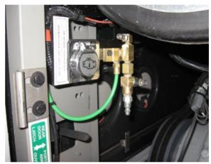
FIGURE 24 : ENGINE COMPARTMENT EMERGENCY AIR-FILL VALVE
