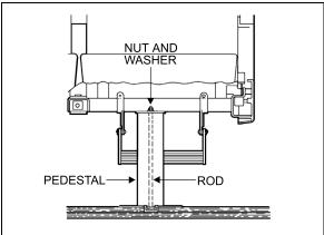
FIGURE 92: SEAT PEDESTAL ASSEMBLY
