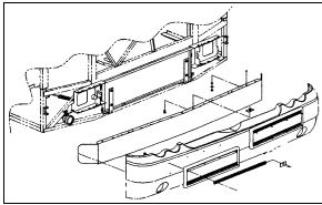
FIGURE 14: FRONT BUMPER REMOVAL 18565
