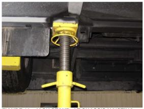
FIGURE 18: JACK STAND AT CHASSIS HOISTING RECEPTACLE - AFT OF FRONT AXLE, ROAD SIDE
