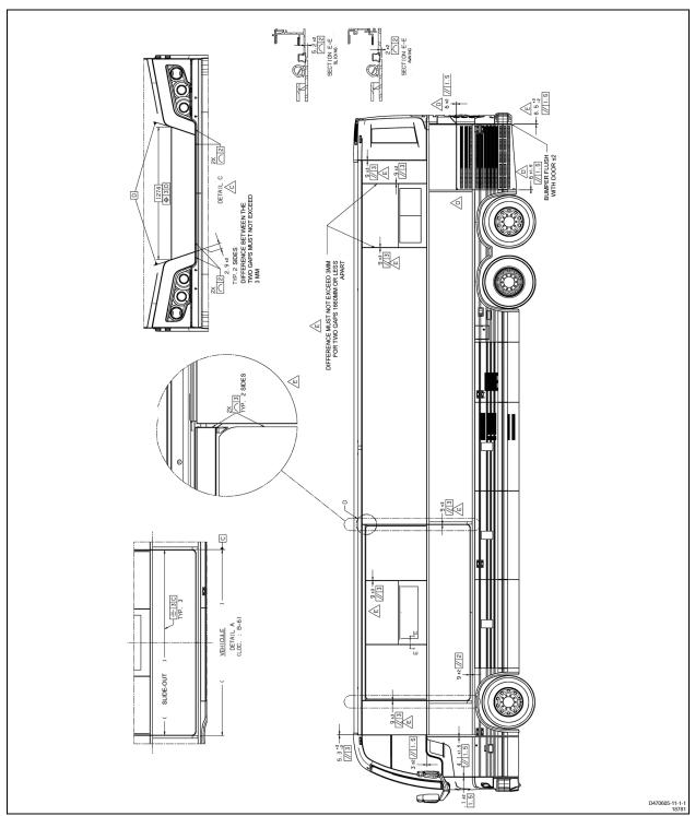
FIGURE 152: BODY PANEL & WINDOW SPACING FOR X3-45 VIP WITH SLIDE-OUT, FRONT
