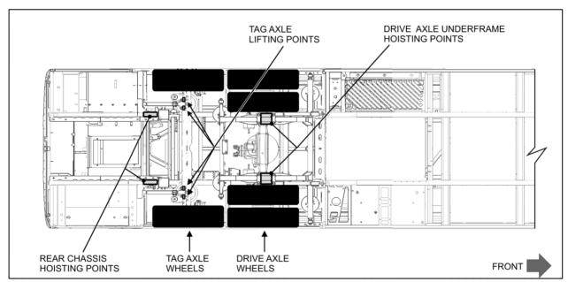
FIGURE 2 REAR HOISTING AND LIFTING POINTS DIAGRAM
