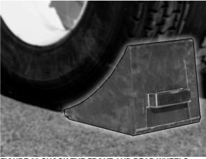
FIGURE 22 CHOCK THE FRONT AND REAR WHEELS
