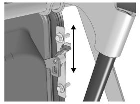
6. Open baggage compartment door and adjust using the cylinder mounting block.
