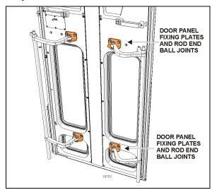
FIGURE 38: DOOR PANEL ADJUSTMENTS
