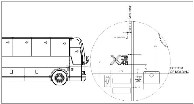
FIGURE 86: SIDE CREST POSITIONING 18639
