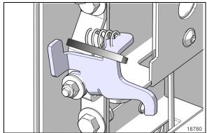
FIGURE 118: USE A CABLE TIE TO KEEP SECONDARY LOCK DEPRESSED DURING ADJUSTMENT
