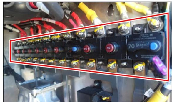
FIGURE 24: DISJONCTEURS PRINCIPAUX DANS LE COMPARTIMENT PRINCIPAL D'ALIMENTATION
