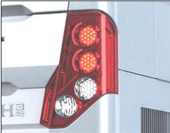
FIGURE 109: MODULE DES FEUX ARRIÈRE – SÉRIE H3
