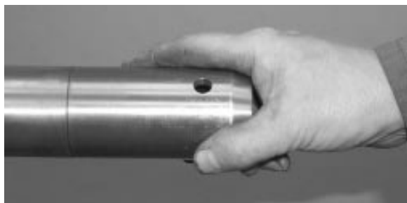
FIGURE 18: OUTIL D'INSERTION N/P PREVOST 491115
