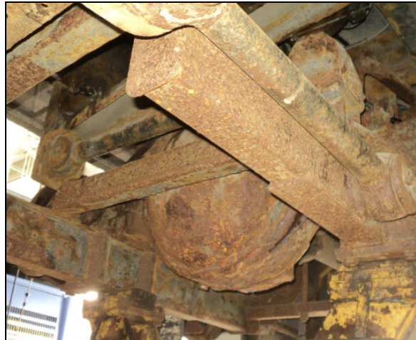
FIGURE 8: NETTOYER LA ROUILLE
