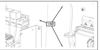
6. Install the new module 23499009-A37 with the screws 500209 (3x) and the washers 500804 (3x).
