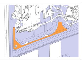
12. Clean the surface of the panel with silicone remover 682989.
