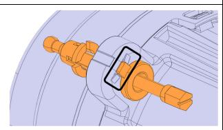
12. Install new lamps 930074(2x) and 930073(2x) with adjuster on the support **(both sides).**
