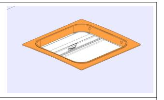
6. Secure the hatch frame with clamps (8x) and use pieces of wood between the clamp and the roof and ceiling finishing as a protection. **The clamps must remain in place for three hours**.
