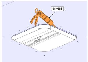
3. Clean the roof panel with silicone remover 682989.
