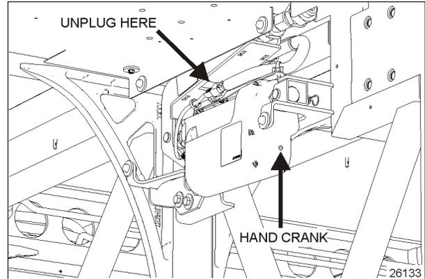
FIGURE 16: MOBILE FLOOR HAND CRANK SOCKET LOCATION
