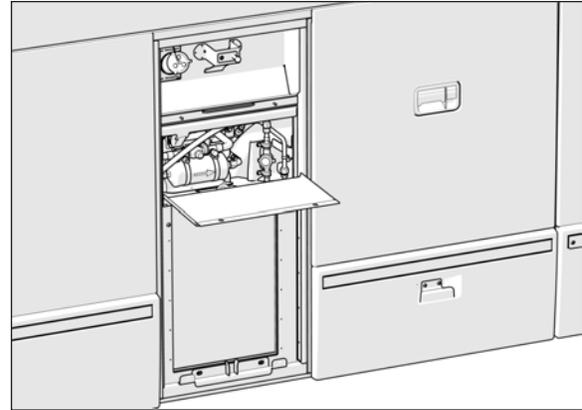
FIGURE 11: A/C CONDENSER COMPARTMENT
