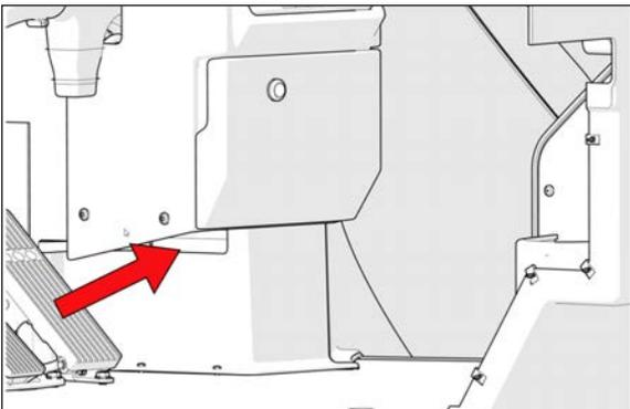
**FIGURE 22: ACCESS TO THE RECIRCULATING AIR FILTERS**
