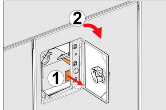
FIGURE 12: A/C CONDENSER COMPARTMENT HATCH OPENING
