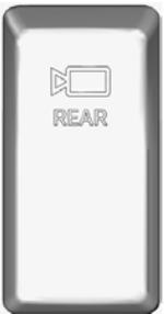
Press down this switch to activate the back-up camera and monitor when the transmission is not in reverse gear.
