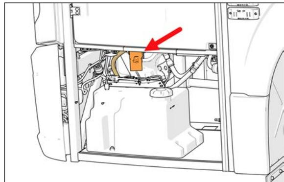
FIGURE 17: WIPERS MECHANISM ACCESS HATCH RELEASE LEVER
