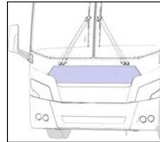
This access hatch can be opened downward to give access to the wipers mechanism. To open:
