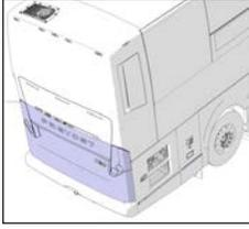
To open the engine door, first open the curbside door. Lift the latch release lever. Unlatch the door and pull it out and up.
