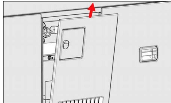
FIGURE 13: A/C CONDENSER COMPARTMENT HATCH OPENING
