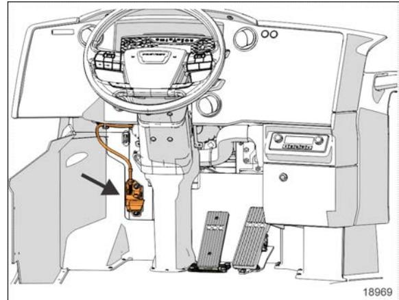
FIGURE 35: STEERING WHEEL TILT AND TELESCOPIC ADJUSTMENT
