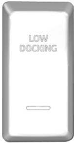
The switch allows lower intensity illumination of the docking lights.
