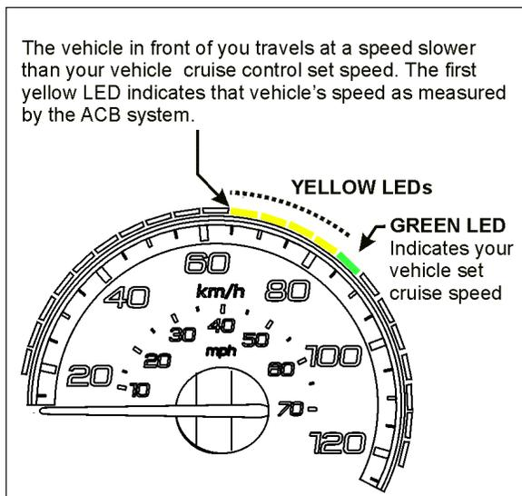
FIGURE 50: EXAMPLE OF THE SPEEDOMETER LED DISPLAY WHEN THE FORWARD VEHICLE IS SLOWER WHILE THE COACH TRAVELS WITH THE ACB CRUISE CONTROL ON AND SET
