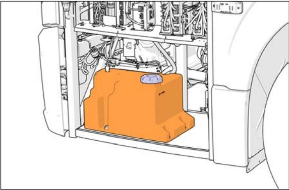
FIGURE 10: WINDSHIELD WASHER FLUID RESERVOIR
