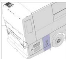
To open the main power compartment door, use the exterior compartment door key. The door will pop open.
