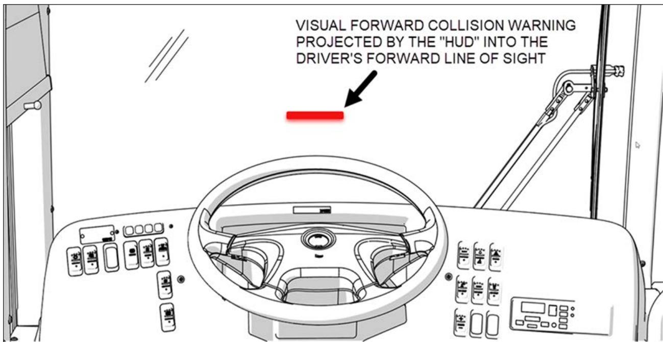
FIGURE 44: HEAD-UP DISPLAY PROJECTED VISUAL WARNING
