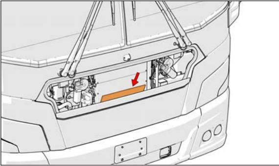
**FIGURE 21: DRIVER HVAC SYSTEM FRESH AIR FILTER**
