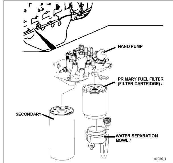
**FIGURE 15: FUEL FILTERS WITH VOLVO D13 ENGINE**
