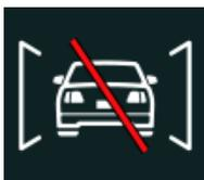
FORWARD VEHICLE DETECTED - MISSING/ERROR STATE pictogram
