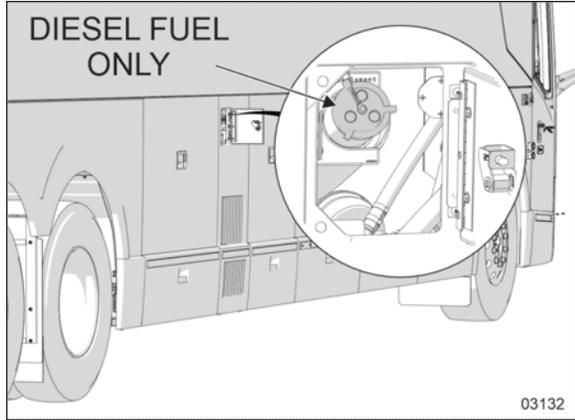
FIGURE 10: CURB SIDE FUEL FILLER NECK ACCESS
