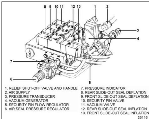
FIGURE 13: PNEUMATIC CONTROL PANEL
