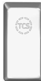
On certain road conditions, it may be useful to retard the intervention of the traction control system TCS during vehicle acceleration. The Mud/Snow function allows greater engine power and more wheel spin during TCS operation. This function may be helpful to set the vehicle in motion on iced roads, for example.
