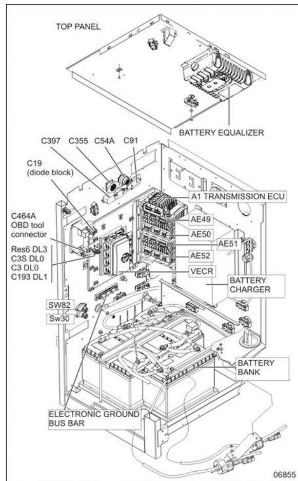
FIGURE 8: VIEW OF MAIN POWER COMPARTMENT (TYPICAL)
