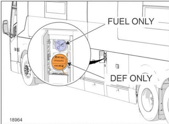
**FIGURE 25: STREET SIDE FUEL AND DEF FILLER NECKS ACCESS HATCH**
