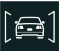
FIGURE 48: FORWARD VEHICLE DETECTED STATUS PICTOGRAM (WHITE)
