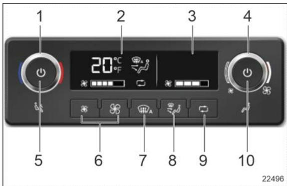
FIGURE 19: DRIVER HVAC SYSTEM CONTROL UNIT WITH AUXILIARY AIR
