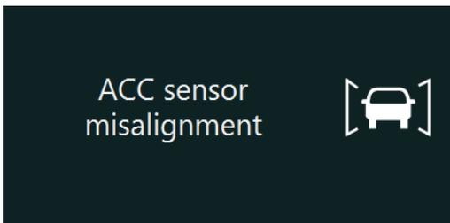
ACB SENSOR (RADAR) FAULT
