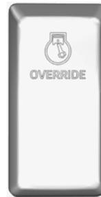
Press the Engine Stop Override switch on the dashboard or the Delay Engine Stop switch on the AFSS protection panel to delay the engine shutdown and extinguisher discharge by an additional 15 seconds.
