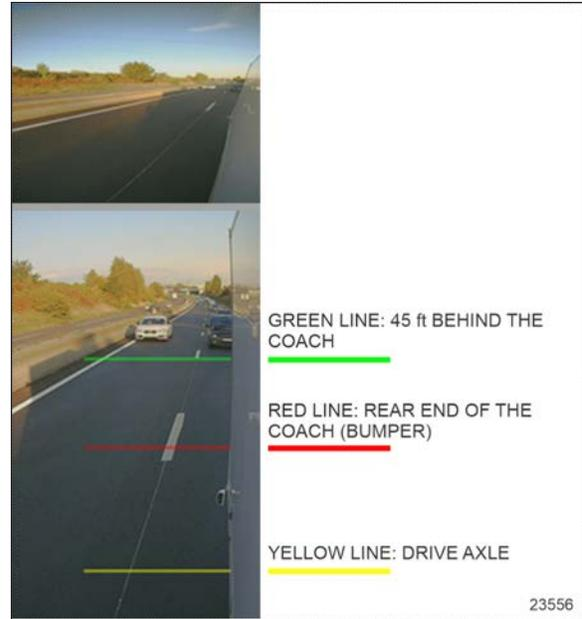
FIGURE 54: REFERENCE LINES IN MONITOR
