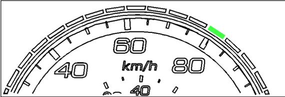
FIGURE 49: THE CRUISE SET SPEED IS 80 KM/H
