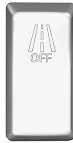
To avoid erroneous LDW warnings in areas such as the work zone where the road markings present might cause false alerts, LDW system can be disabled by the driver using the enable/disable switch. LDW system will reactivate automatically after a delay of 15 minutes or a transition from OFF to ON of the ignition or upon pressing of the enable/disable switch a second time
