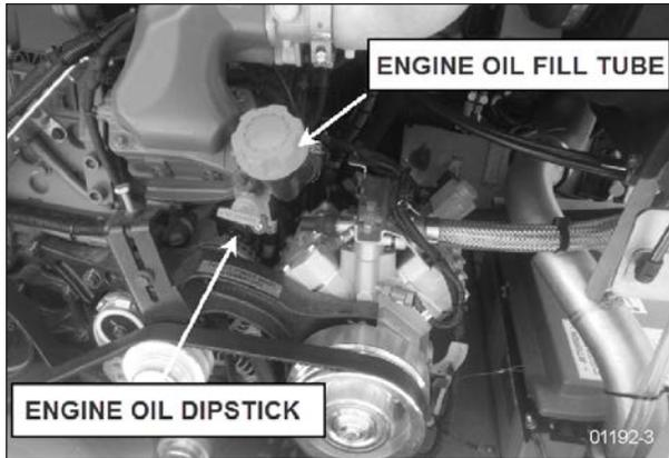
FIGURE 1: ENGINE OIL DIPSTICK - VOLVO D13 ENGINE
