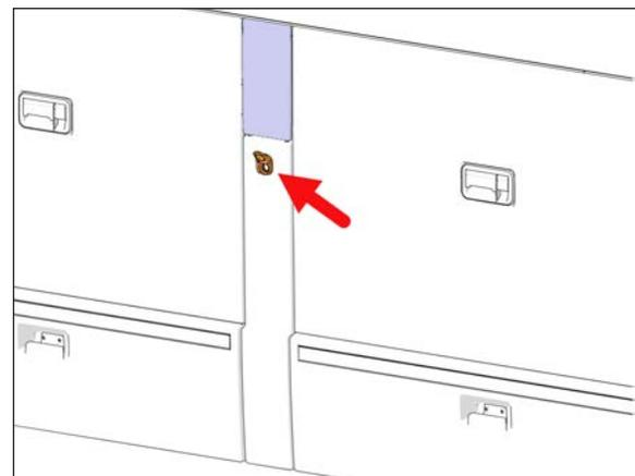
**FIGURE 24: FILLER NECKS ACCESS HATCH LOCK**
