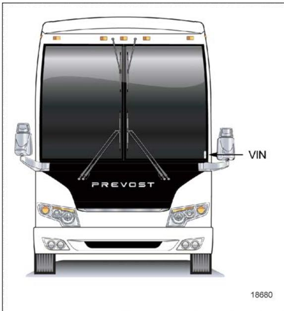
**FIGURE 8: VEHICLE IDENTIFICATION NUMBER (H3 SERIES)**
