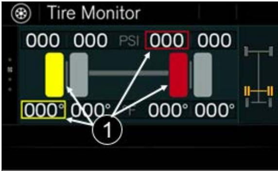
FIGURE 37: READING PRESSURE AND TEMPERATURE ON DRIVE AXLE TIRES WITH IRREGULARITIES DETECTED (DISPLAY EXAMPLE)
