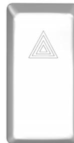
Press the rocker switch to make all turn signal lights flash at once. The dashboard telltale lights will flash when the hazard warning flashers are ON.
