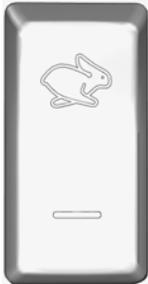
For extended idling periods, run the engine at fast idle. Press down this rocker switch to engage fast idle. This increases the engine speed to approximately 1,000 rpm. Return to normal idle before driving or when stopping the engine.
