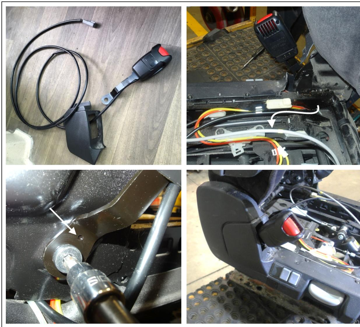
5. Install new seat belt and mechanism.
