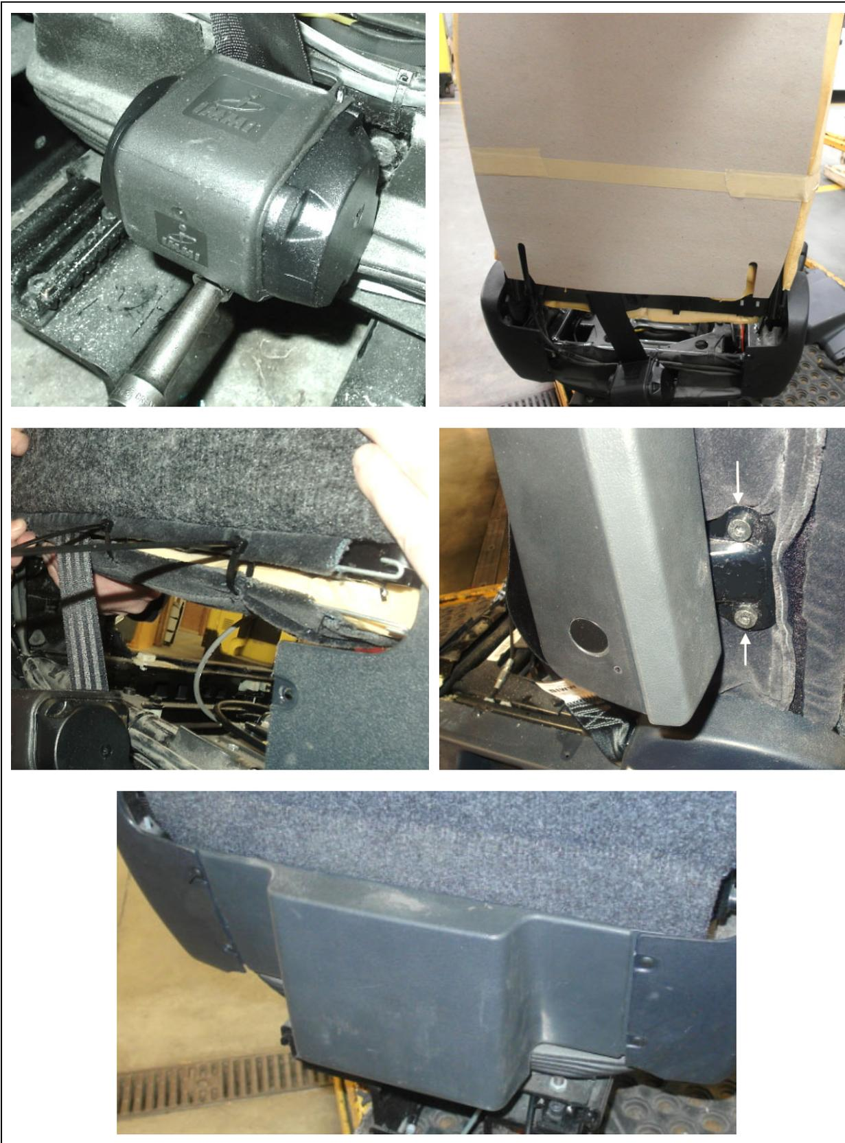
6. Connect the buckle harness to the vehicle.
