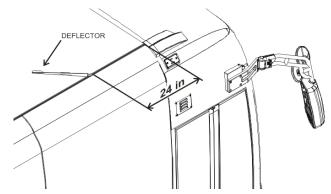
Using isopropyl alcohol or Sika cleaner, clean the roof surface and deflector where Simson sealant adhesive will be applied and allow drying.
