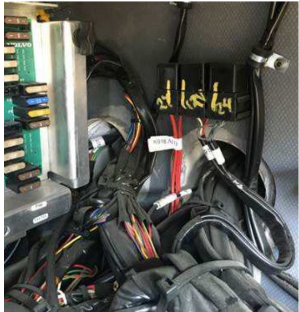
FIGURE 4: For vehicles not equipped with I-START dual battery system (until 3CET2V42XG5176275 ), find K918 at the right side of electrical distribution unit.
