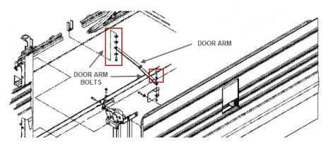
5. Install the new shorter door support arm following hardware stacking order below at the structure point.
