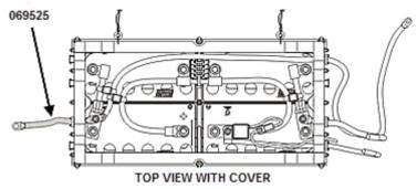
**5.** Secure the cable at the terminal end and chassis ground stud. Torque nuts to **170 lb-in.**
