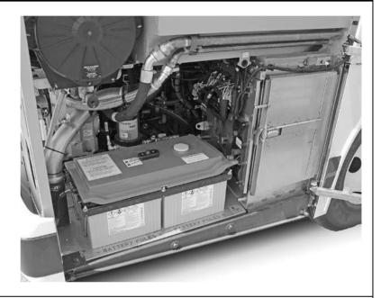
2. Locate the **069525** ground cable connected to the chassis ground stud (left side; see image).
