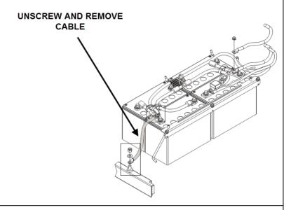
4. Replace the cable with the supplied 069525 cable.
