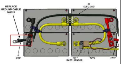
3. Disconnect the cable at the battery terminal and chassis ground stud. Remove the cable from the vehicle.
