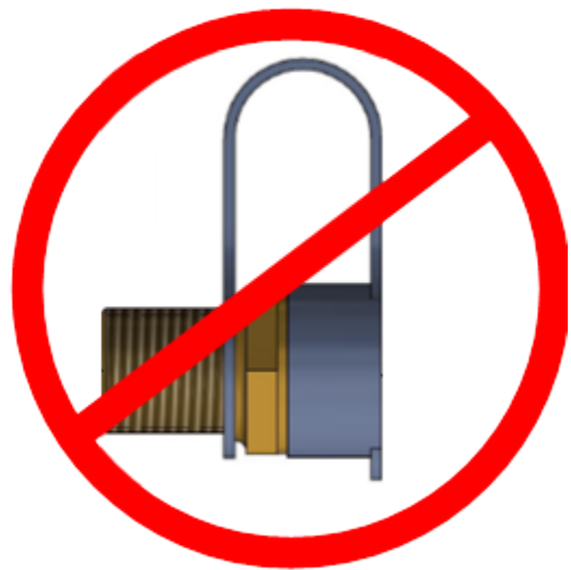
WRONG LOOP POSITION
