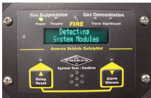
Identifies Number of Modules Found (Driver, Detection, Detection Release, and/or Release Module)
