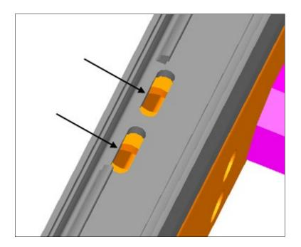
4. If the holes are misaligned, use a 1/2in (13mm) hollow punch to puncture the seal & relieve the drain holes. Apply hand pressure and twist from left to right to cut through the seal.
