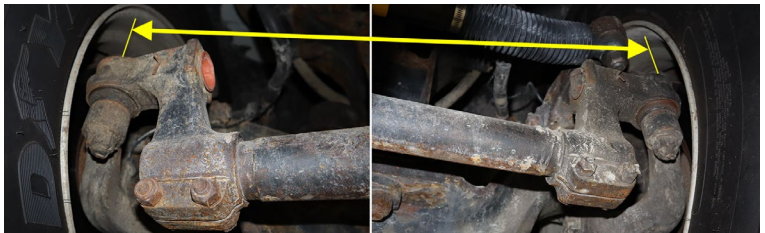
FIGURE 3: TIE ROD BALL JOINT CENTER TO CENTER MEASUREMENT
