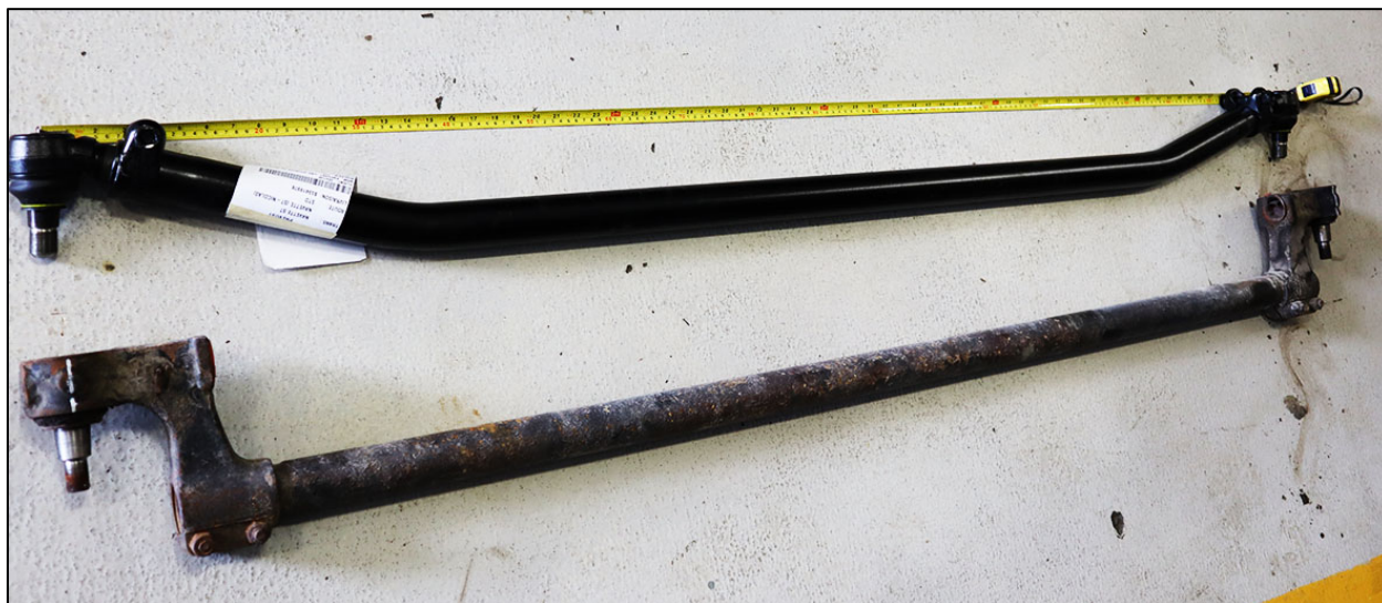
FIGURE 1: OLD TIE ROD ASSY VS NEW ABOVE
