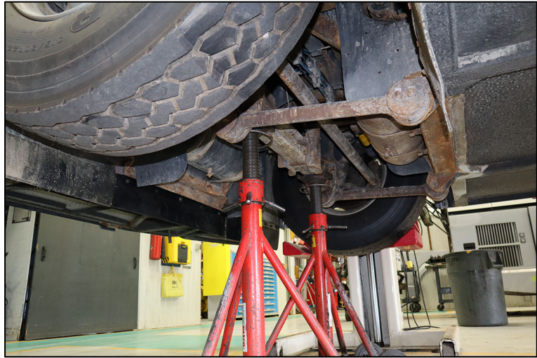
FIGURE 2: JACK STANDS PLACEMENT
