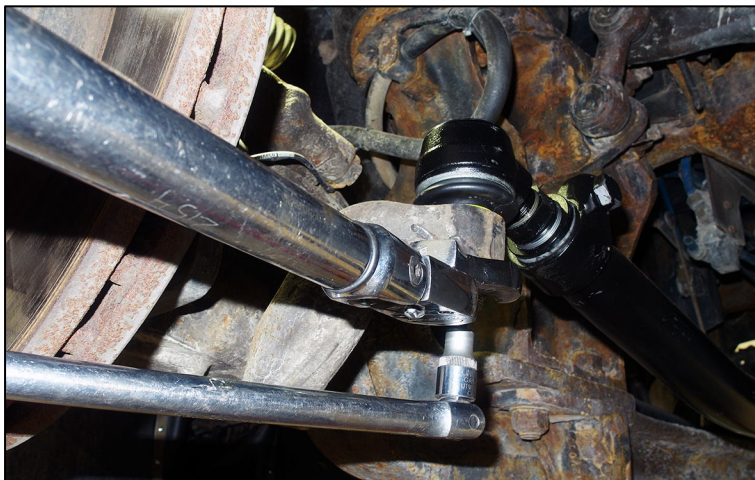
FIGURE 11: BALL JOINT TIGHTENING
