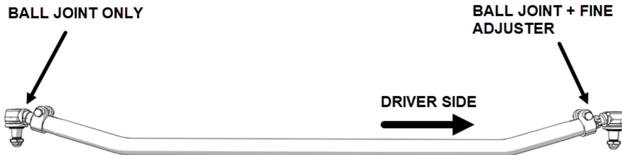
FIGURE 6: TIE ROD ASSEMBLY - 2 DIFFERENT BALL JOINT ADJUSTMENT TYPES
