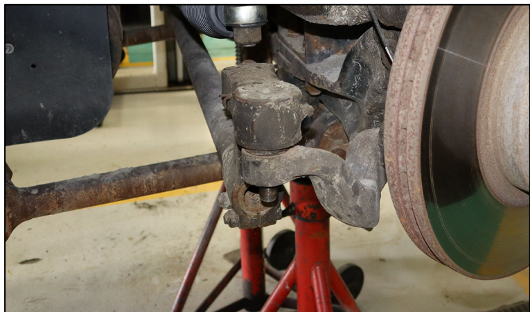
FIGURE 4: BALL JOINT DISASSEMBLY
