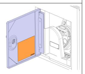
9. Install the new fuel tank capacity decal 406966 on left side fuel door at indicated position.
