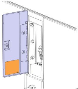
9. Install the new fuel tank capacity decal 406966 on left side fuel door at indicated position.
