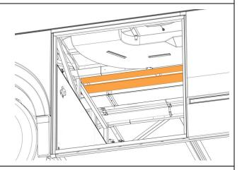
3. Locate the structure tube to which PVC pipes will be attached inside the first baggage compartment.
