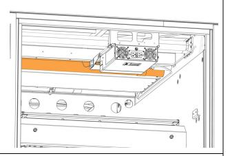
5. Locate the structure tube to which PVC pipe will be attached inside the fifth baggage compartment.
