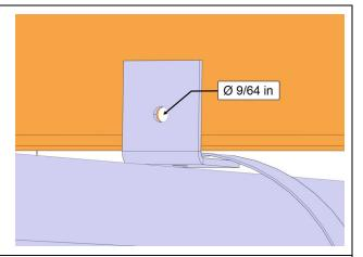
8. Fasten the support to the structure tube with screw 500957 to secure pipe.
