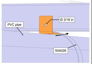
6. Tighten the hose clamp to secure support in place.
