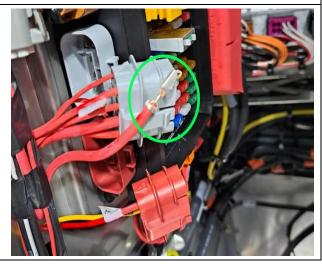
13. Insert the terminal at position **G** of the connector **VECR1** (gray)
