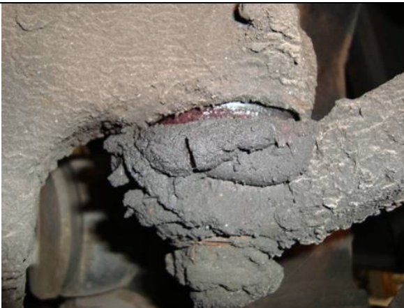
BEFORE- REMOVE OLD GREASE
