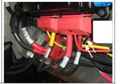
Secure cable bundle at arrow locations making sure to clear the heat sink of the nearby Multiplex module.
