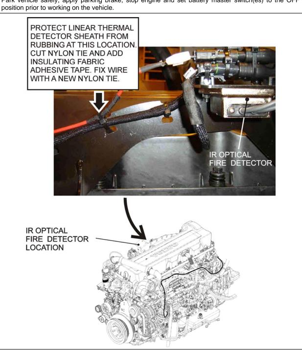
1. There is only one location where the protective fabric tape might be too short or improperly located. Check the engine turbocompressor side near the optical infrared (IR) fire detector (see image above).
