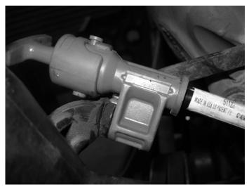
5. Fill tube will need to be rotated slightly away from new dipstick handle.
