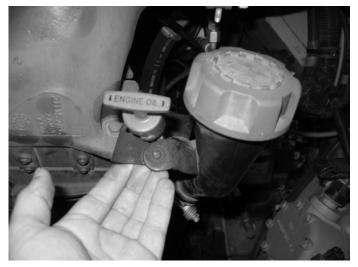
8. Make sure there is no remaining tension on the fill tube before tightening the collar and clamp.
