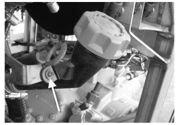
3. Follow the dipstick tube towards the oil pan and remove all clamps and one double loop cable tie.
