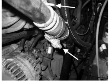
7. Rotate fill tube to this suggested position.
