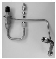
7. Install 5011082 tube compression fitting on the bare end of the bypass tube welded assembly.
