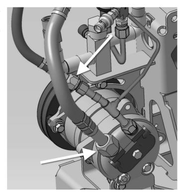
12. Support by-pass valve to alternator bracket with P-Clamp and provided hardware.
