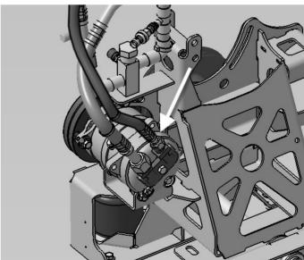
4. Disassemble Low pressure sensor. Keep for re-assembly.
