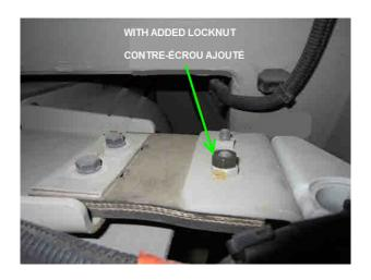
ALL TYPES. Add two locknuts #502851 as described on the image at right. If needed, tighten the bolt a little bit more to show more threads.
