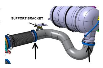
ALL TYPES. Add two locknuts #502851 as described on the image at right. If needed, tighten the bolt a little bit more to show more threads.
