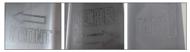
5. Slide the new condenser between the brackets and the radiator and secure in place using appropriate hardware with the condenser connections facing the *front* of the vehicle.
