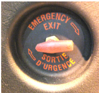
FIGURE 4: INTERIOR EMERGENCY DOOR OPENING VALVE
