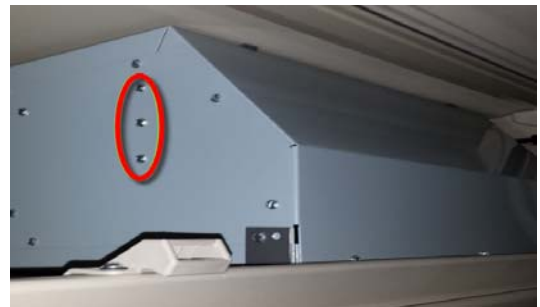
Insert the 2 nd sensor in the defrost return air intake, under the screw found at the center.
