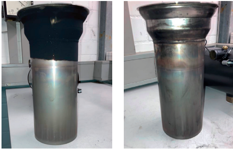
Combustion chamber before ... and after cleaning.
