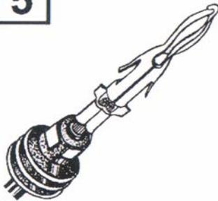
HAND CRIMP CORE WINGS FIRST, THEN INSULATION WINGS USING ONE OF THE APPROVED CRIMPING TOOLS. USE CRIMP MATRIX IN THE TABBED SECTIONS TO DETERMINE CORRECT TOOL COMBINATION.
