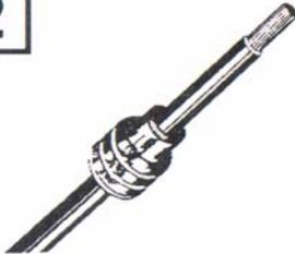
APPLY CORRECT SEAL PER GAUGE
