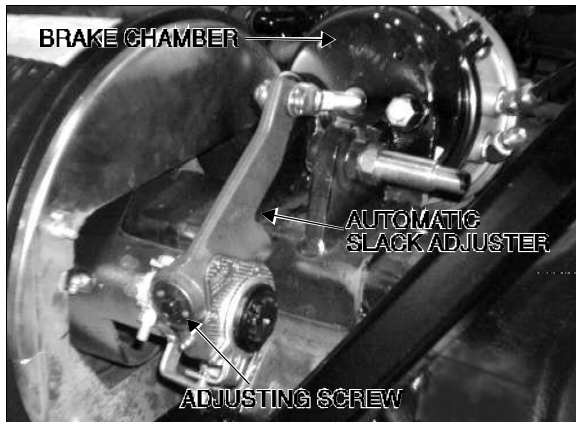
FIGURE 14: DRUM BRAKE ASSEMBLY 12044
