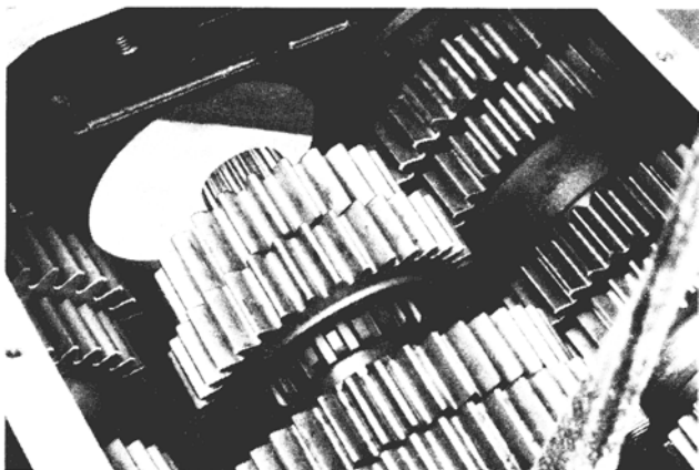
21. To provide necessary clearance for mainshaft removal, move both countershafts forward and toward the side of the case. Countershaft alignment blocks can also be used to help restrain the countershafts.
