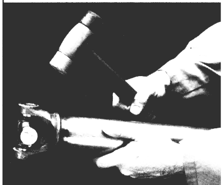
5. Repeat steps 3 and 4 to install the opposite bearing assembly. If the joint is stiff, strike the yoke ears with a soft hammer to seat the needle bearings.
