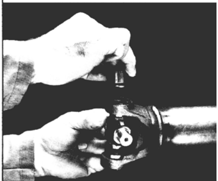
5. Repeat steps 3 and 4 to install the opposite bearing assembly. If the joint is stiff, strike the yoke ears with a soft hammer to seat the needle bearings.
