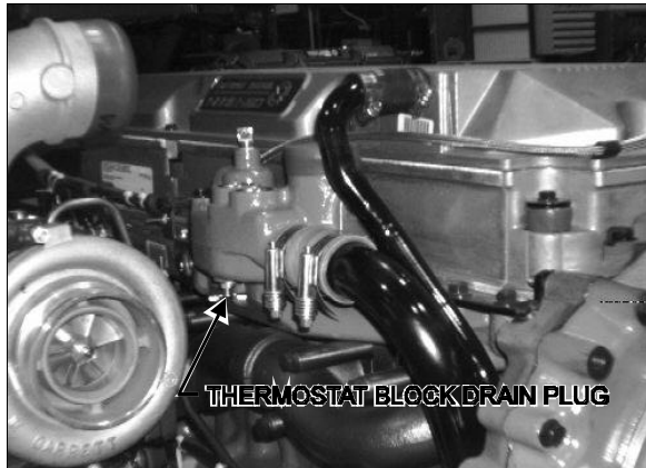
FIGURE 9: THERMOSTAT BLOCK DRAIN PLUG 05029
