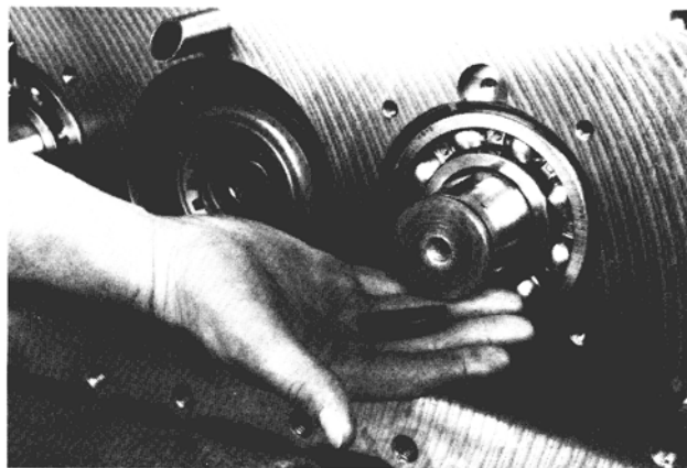
11. Continue by removing the countershaft driver gear countershaft keys.
