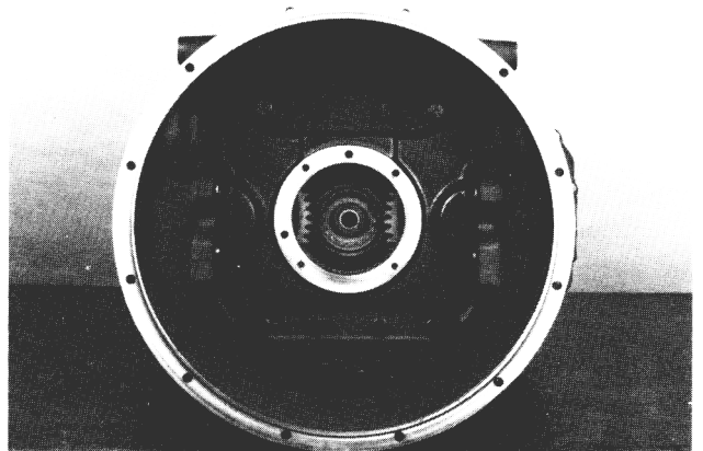
18. Apply a light coat of Loctite 51 5 to the clutch housing. Attach the housing to the case and secure it with capscrews. Torque them to 150-180 ft. lbs.
