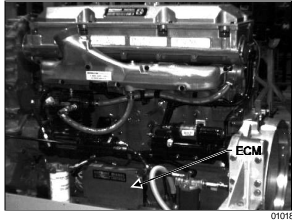
FIGURE 2: ELECTRONIC CONTROL MODULE (ECM)
