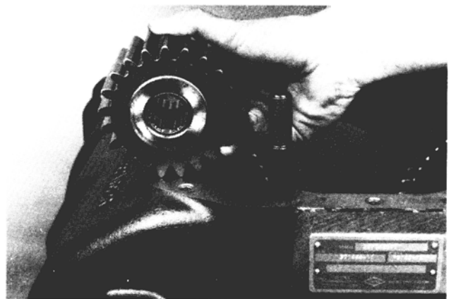
23. Remove the upper reverse idler gear.
