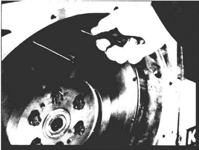
Insert two 7/16" - 14 UNC (5" long) guide studs into the two upper mounting holes of the flywheel.
