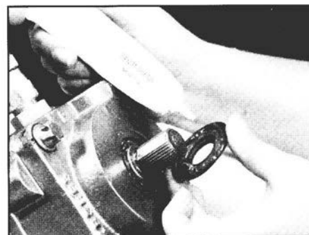
Install dirt & water seal
